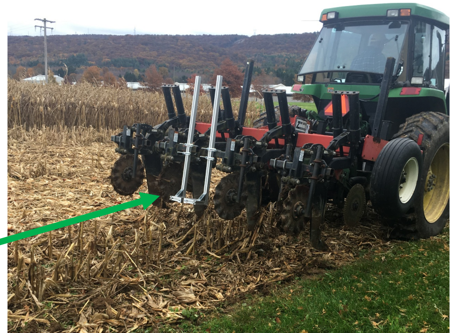
Field test for stalk guide bars (Stalks stay straight up after being deeply tilled and guided)
